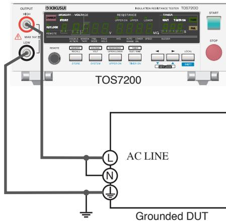
Fig.3-6 Connecting the Tester to a Grounded DUT (insulation resistance test across the AC LINE and chassis of the DUT)
