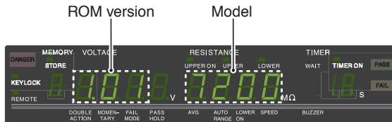
Fig.3-1 Example of Display of the Version Number
