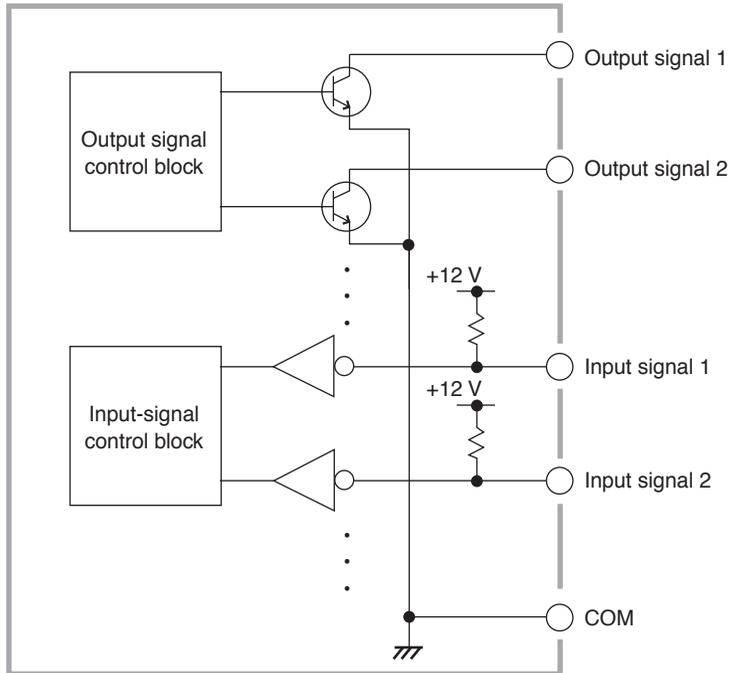
Fig.4-3 Internal Configuration of the SIGNAL I/O Connector
