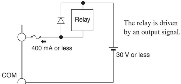
Fig.4-6 Example of Driving the Relay
