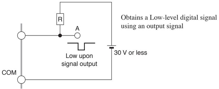
Fig.4-7 Example of Obtaining a Low-level Digital Signal
