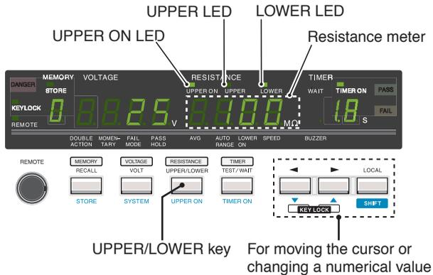
Fig.3-3 Setting a Lower Resistance
