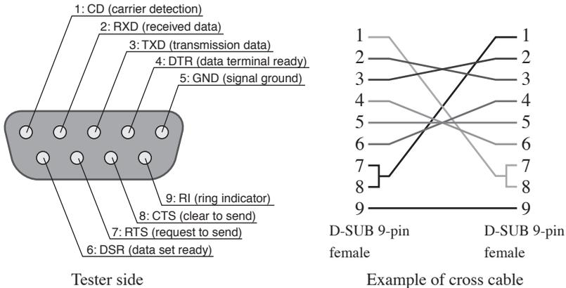
Fig.5-1 9-pin AT-type Connector
