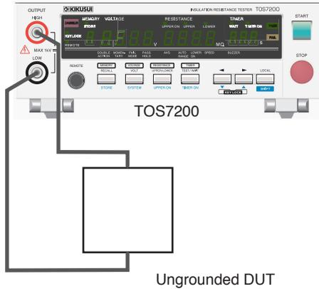
Fig.3-7 Connecting the Tester to an Ungrounded DUT
