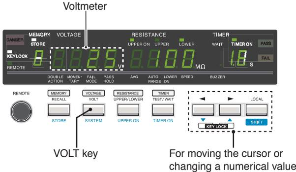
Fig.3-2 Setting the Test Voltage
