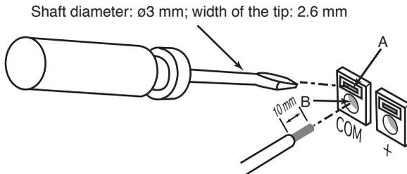
Fig.4-10 Connecting a Signal Wire to the ANALOG OUT Connector
