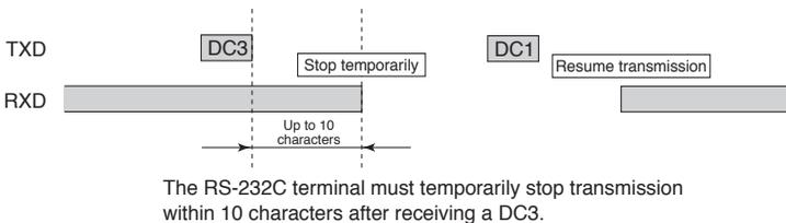
Fig.5-2 Transmission Control between the RS-232C Terminal and Tester
