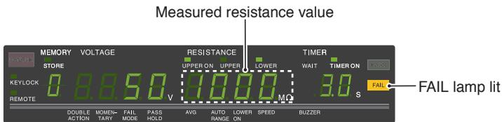
Fig.3-11 Example of the Display for FAIL Judgment
