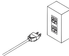
Grounded three-contact electrical outlet
