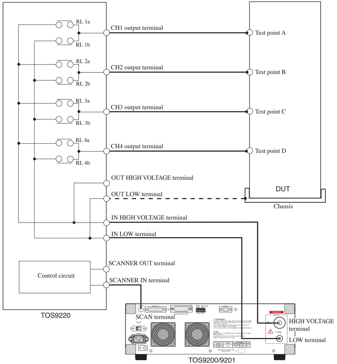
Fig.3-5 Test System 2 Using the TOS9220 Scanner
